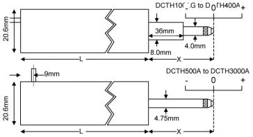
Our spring displacement transducer has bearings to guide the armature inside the measurement sensor and a spring which pushes the armature to the fully out position. Spring return LVDTs are appropriate where it is not possible to connect the transducer armature to the moving component being measured.
