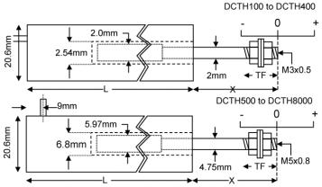
On our unguided LVDTs the armature assembly is a separate component, to make a measurement the user must guide the armature inside the body without touching the sides. Unguided position measurement transducers are appropriate where external guidance is available and give truly non-contact operation
